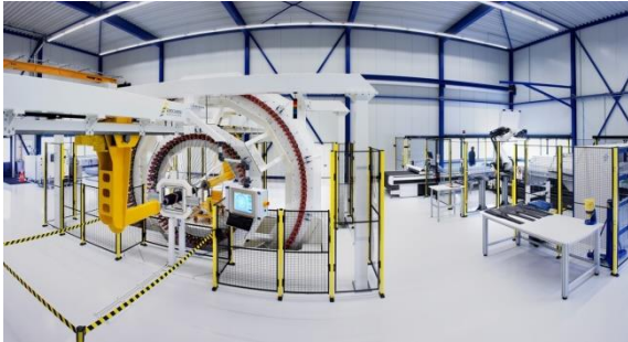
Fig. 4: The Automated Composite Manufacturing Pilot Plant, showing the RTM facility at far left, an overbraiding facility at left centre, and a raw material pick & place and automated preforming facility at the right (NLR)
